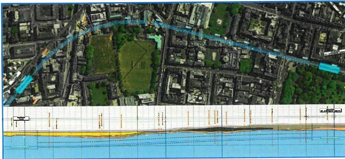
Figure 6. Geological Section (ref. A5.13, Diagram 3.13: Geologic Profile for TBM Drive C8- Tara Station to St. Stephen's Green)
